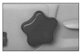
If your vehicle has this feature, the knob is located on the outboard side of the driver's seat. Turn the knob toward the front of the vehicle to increase lumbar support. Turn the knob toward the rear of the vehicle to decrease lumbar support.
